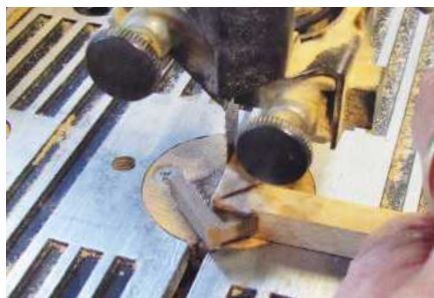
▲ Pic D. Once the glue has dried, it’s simple to trim off the wings of each spline on a bandsaw, then sand the corner smooth. Thanks to modern glues, the finished joint is stronger than the surrounding wood
